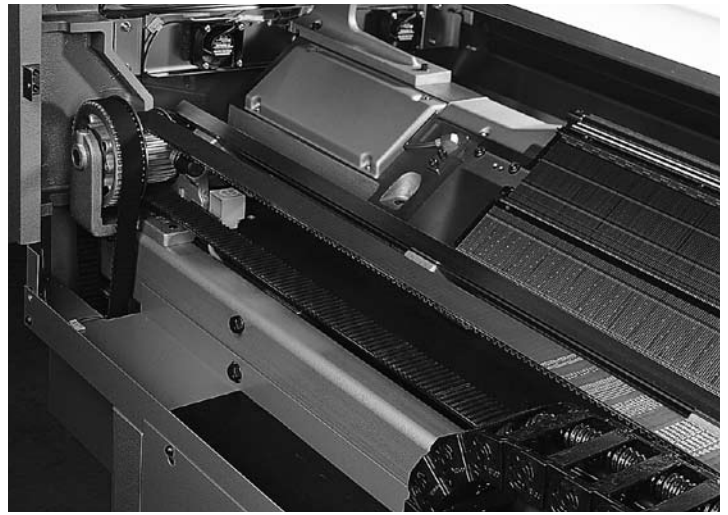
Large Knitting Machine (SUPER TORQUE Timing Belt)
